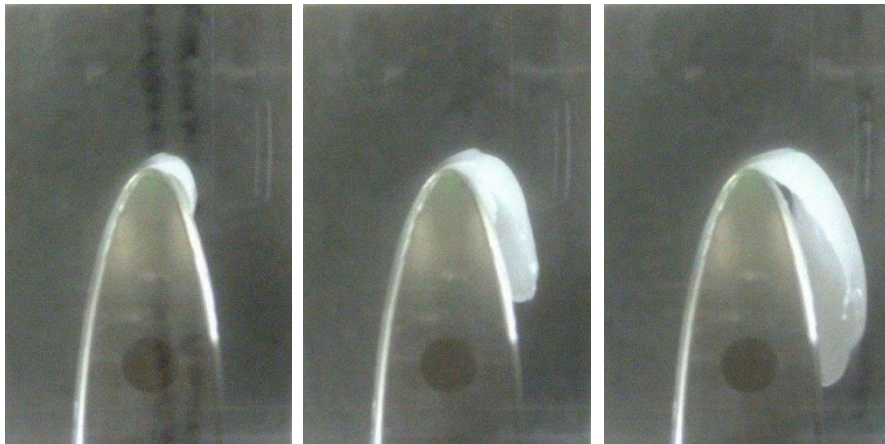
Figure 9. Asymmetric ice shape evolution observed during Test Point 1.02, Scan 917 ( M=0.25 , T_0 = 15^\circ\text{C} , P_0=5 psia, large PSD, T_{wb_0} = 6^\circ\text{C} ). This data was not analyzed.
