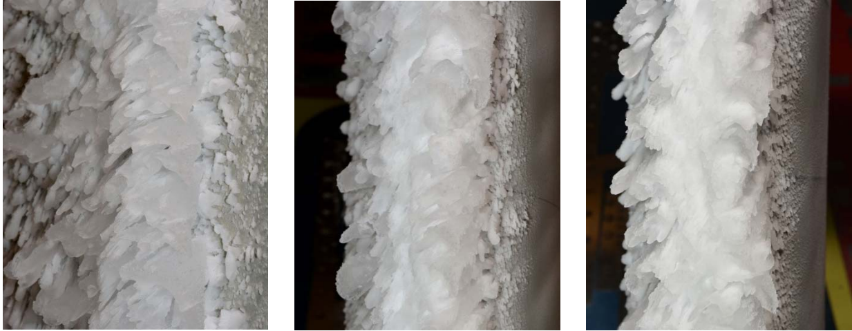
Figure 6. Photographs of Incomplete Scallop ice shape on Inboard (left), Midspan (middle) and Outboard (right) models.
