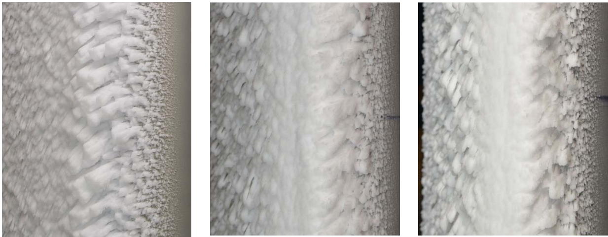
Figure 7. Photographs of Streamwise/Rime ice shape on Inboard (left), Midspan (middle) and Outboard (right) models.
