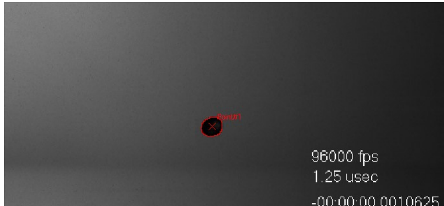
Figure 8. Example of particle tracking software. Software determines edges based on grey scale and calculated center of mass.
