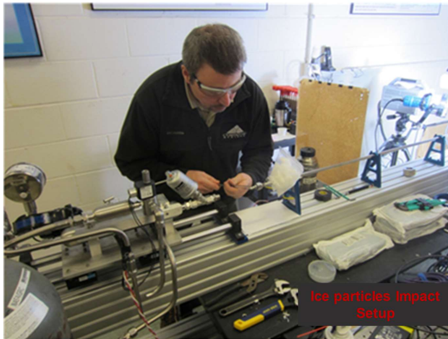
Figure 4. Pressure Gun Main Components. The pressure tank, the solenoid valve, the breech and the barrel are shown.
