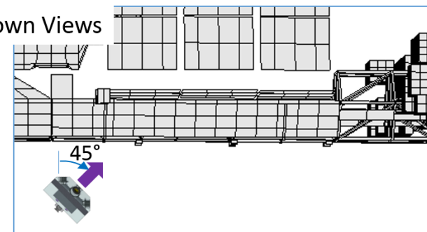
Measurement 3: Rotate the RELL another 22.5° in the port/outboard direction (-Y) maintaining 2 feet clearance from Face 1
