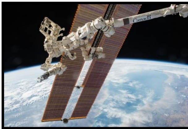
Figure 2: RELL attached to the SSRMS/SPDM during the Technology Demonstration in December 2016.
