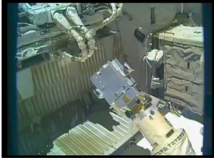
Figure 7: A screenshot of RELL scanning RBVM P1-3-2 as taken from the mast camera of the SSRMS.
