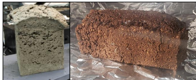
Fig. 16 Left, OPC and martian regolith simulant cured in a CO 2 atmosphere at 7 torr and 20°C (photo included with permission from J. Edmunson). Right, sodium silicate and martian regolith simulant cured in a vacuum at approximately 20°C (image used with permission from J. Amar). Note large vesicle and crack formation due to the escape of water.
