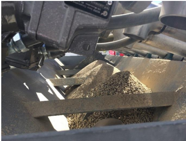
Fig. 10 Dry Goods in Weigh Hopper. Image used with permission from R. Mueller.
