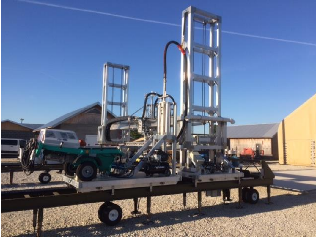
Fig. 7 ACES-3 System Pump/Accumulator Trolley
