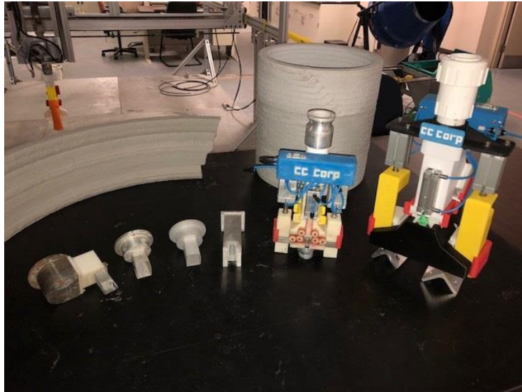
Fig. 5 ACME Nozzle Evolution – single and multiple output nozzles
