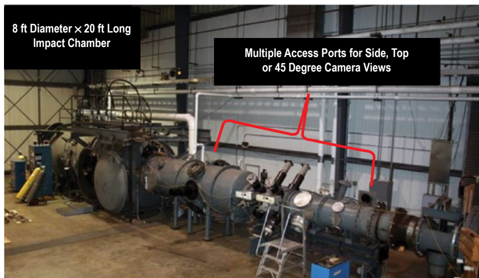
Figure 45. Multiple data acquisition and image access ports for flexible test setup.
