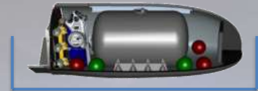
Lander 4 Habitat volume reconfigured to horizontal orientation
