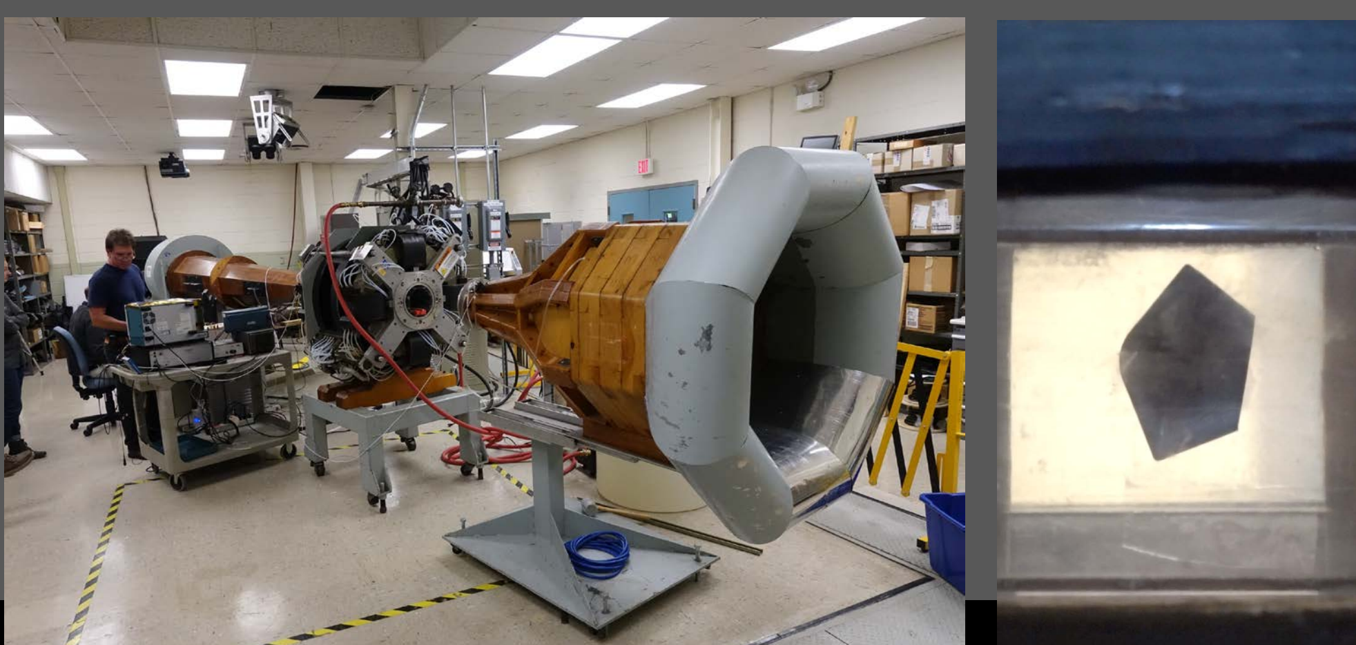
Magnetic suspension wind tunnel and levitation demo
