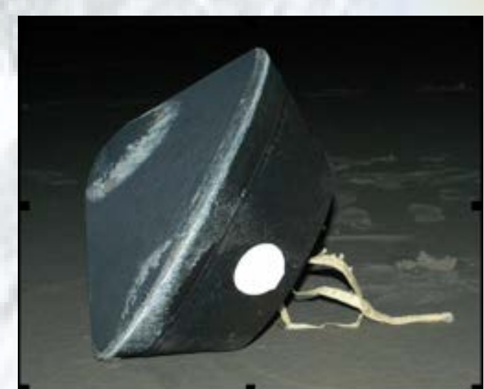
Stardust SRC post flight with PICA forebody heat shield (0.8m max. diameter)
