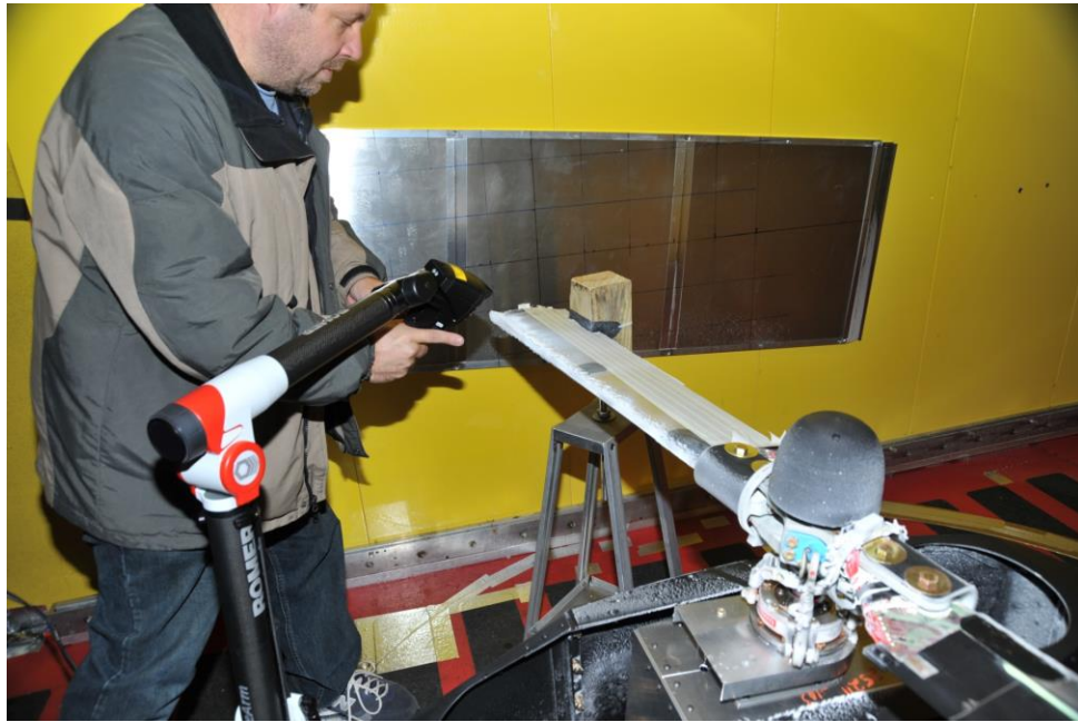
Figure 3. Scanning the Ice on a Tail Rotor in the IRT
