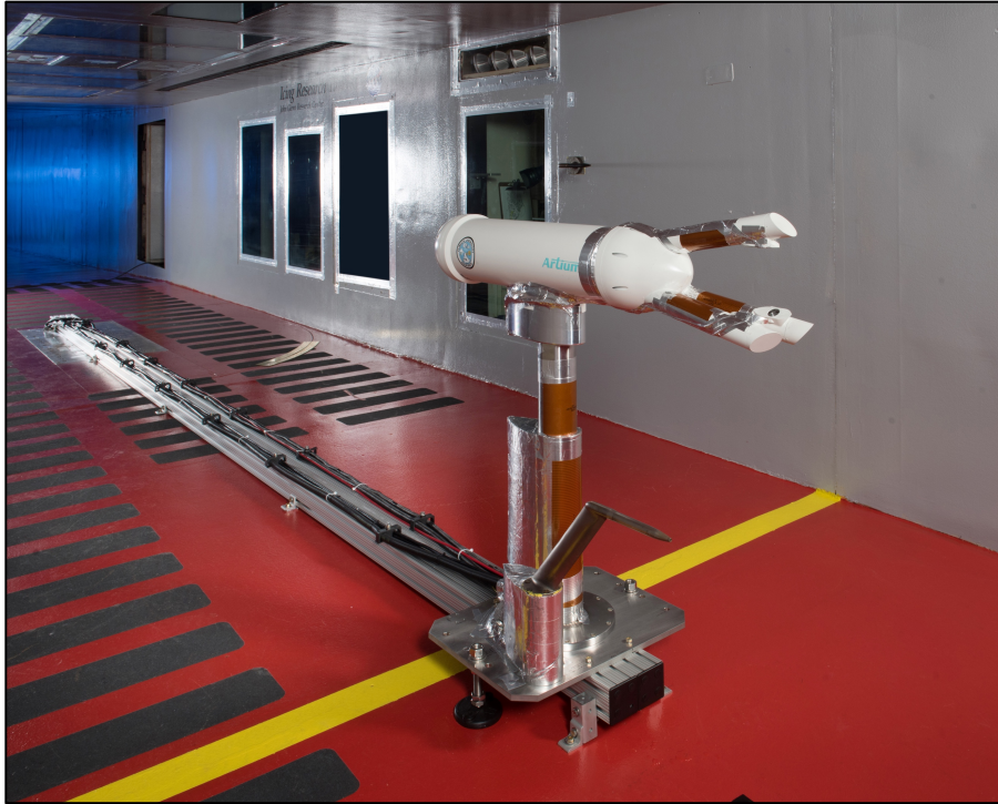
Figure 1. Artium Technologies, Inc. PDI-FPDR and pitot-static probe mounted upstream in the IRT contraction
