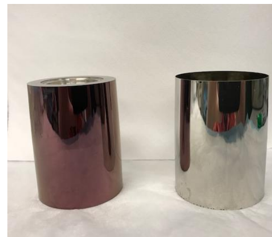
Mandrel ( left ) and replicated NiCo optic ( right )
