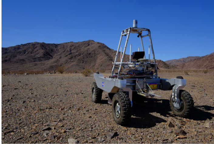
Fig. 1: KRex2 in the Mojave Desert. KRex carried a Neutron Spectrometer System(NSS) and a Near Infrared Visible Light Reflectance Spectrometer (NIRVIS). The robot autonomously drove and localized itself at the command of remote scientists. The data that it collected was georegistered and presented to the backroom of a team of 30 scientists who adapted their plans in response to data updates.
