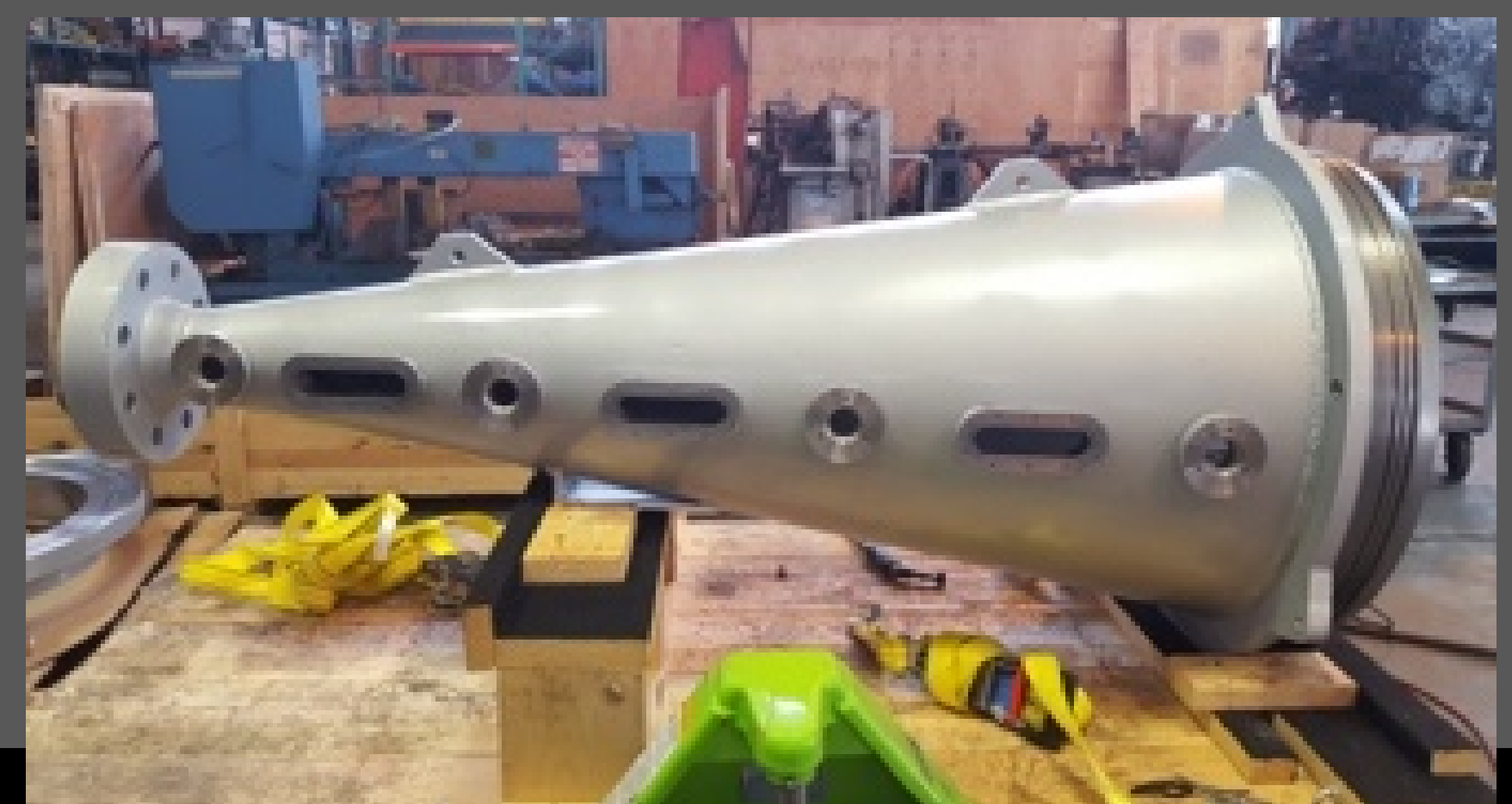
EAST expansion section is installed and ready for testing in Sep/Oct
