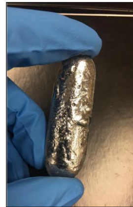
Figure 2. FeSi6 (6 wt.% Si) made in arc melter under Ar.
