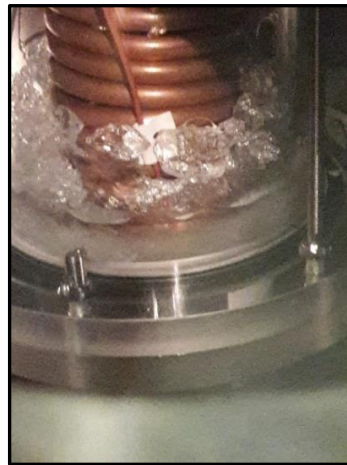
Figure 3. Liquid water forming and pooling at 80 torr and 3°C from ice introduced under Mars surface conditions
