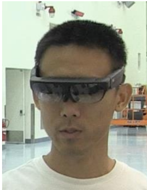
Figure 10 Ground Operations Technician wearing IDEAS compatible Smart Glasses
