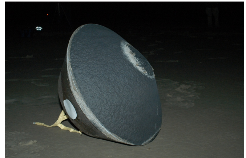
Stardust single piece, seamless heatshield
