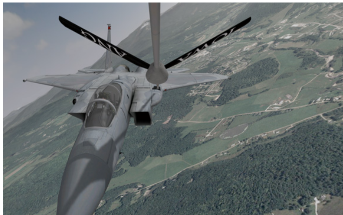
Figure 8. Simulated aerial refueling scene. The shadow of the boom on the aircraft provides an important relative depth cue for the boom operator. Image generated by MetaVR's Virtual Reality Scene Generator™ (VRSG™).
