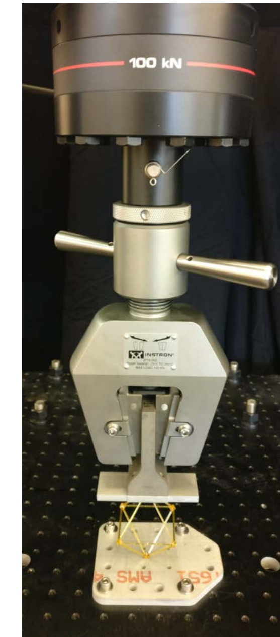
Instron Setup Ultem 1000 Single Voxel
