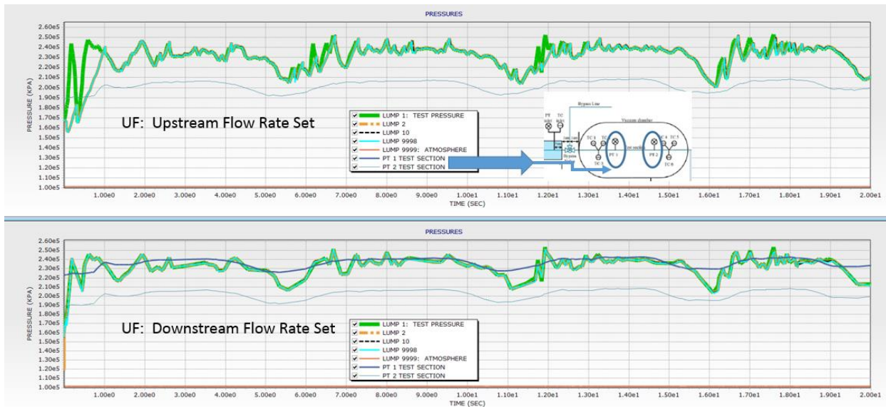
Figure 15: Horizontal Liquid Nitrogen Chill-down (17b) UF Heat Transfer with Pressures through the Test Section (Upstream and Downstream Flow Rate Boundaries)
