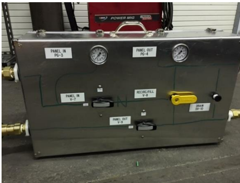
Figure 19: Deionized (DI) water portable panel.
