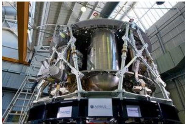
Figure 3: Orion European Service Module (ESM) test article.
