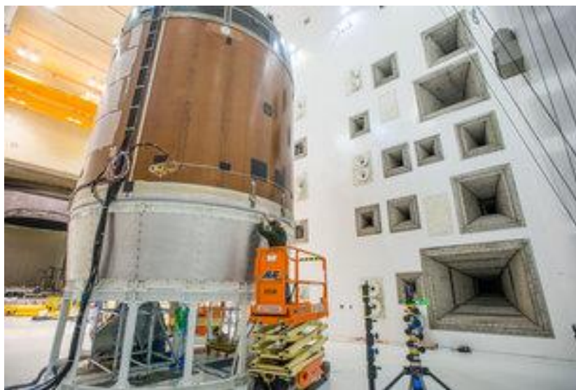
Figure 8: Orion Service Module (SM) test article acoustic test.
