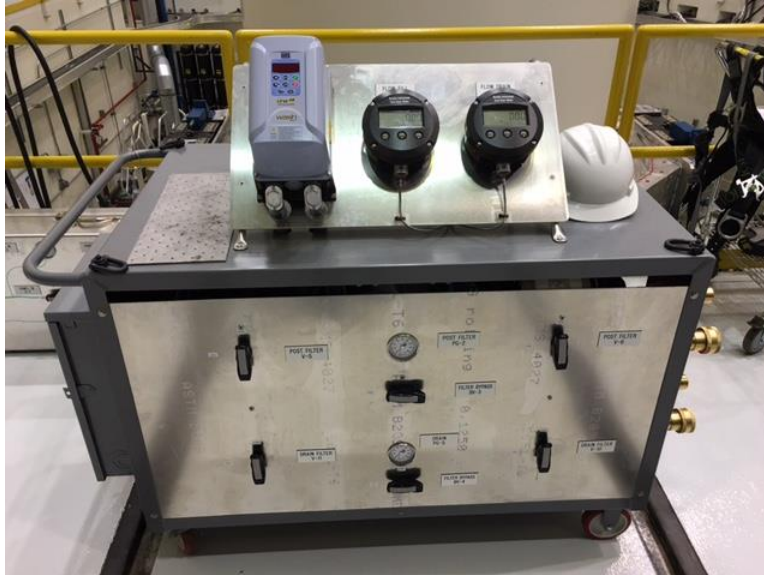
Figure 18: Deionized (DI) water fill and drain cart.
