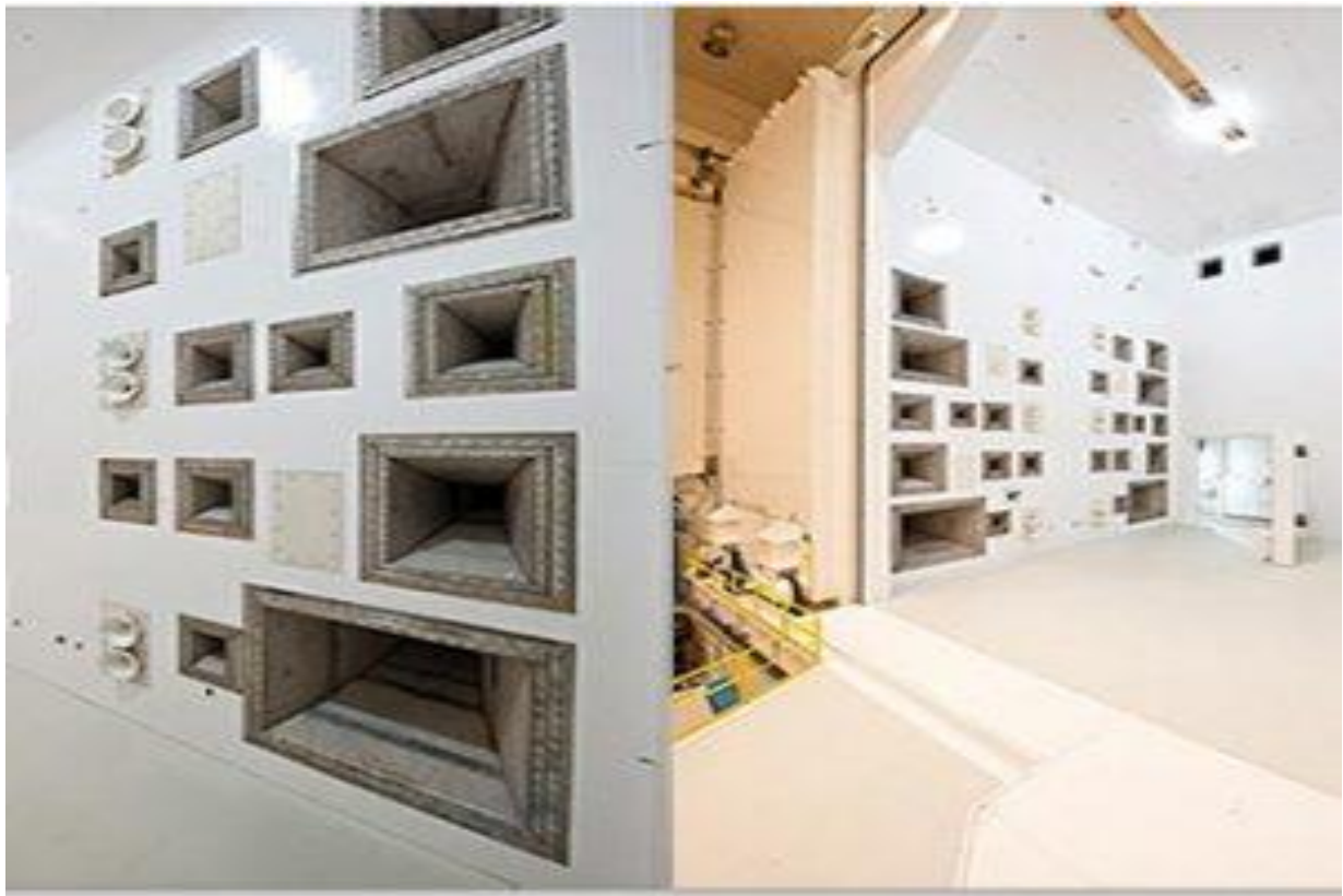
Figure 10: Reverberant Acoustic Test Facility (RATF) horn wall is shown at left, and the overall chamber is shown at right.
