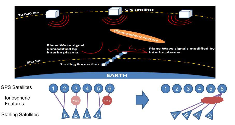
Autonomously reconfigure the spacecraft attitude and channel selection/sampling to improve signal strength and resolution of feature image
