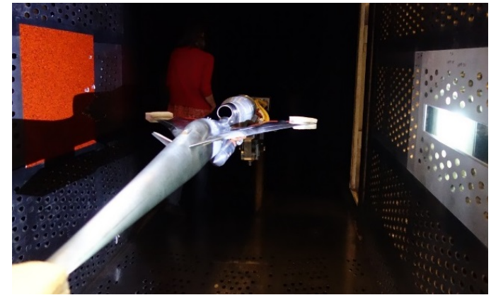
BOS installed in 8x6 SWT for QueSST
