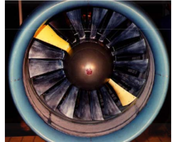
Painted Blades for pressure measurements
