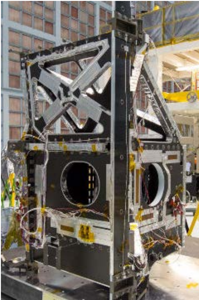
Flight Structure with Thermal Hardware Installed and Earth Shield Hinges and Strong Back
