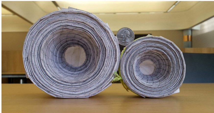
Figure 3.13. Crease pattern that stows to 1/40th of its longest dimension. A 1/16 scale model of an elliptic reflector was also folded demonstrate how it stows and deploys. Partially deployed origami ellipse (top) and same ellipse stowed (bottom). Ellipse is 106 cm × 183 cm.
