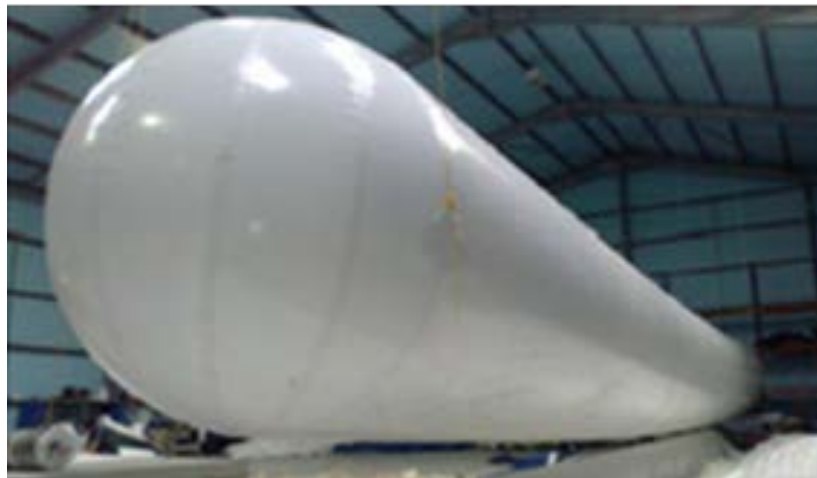
Figure 3.18. 2-m diameter inflatable beam (Photo courtesy Tectoniks).
