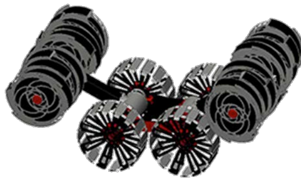
Figure 2.12. KSC excavator RASSOR II, which is the current baseline for the case study. This technique enables the harvesting of large amounts of regolith on a low gravity body with a very low-mass vehicle.
