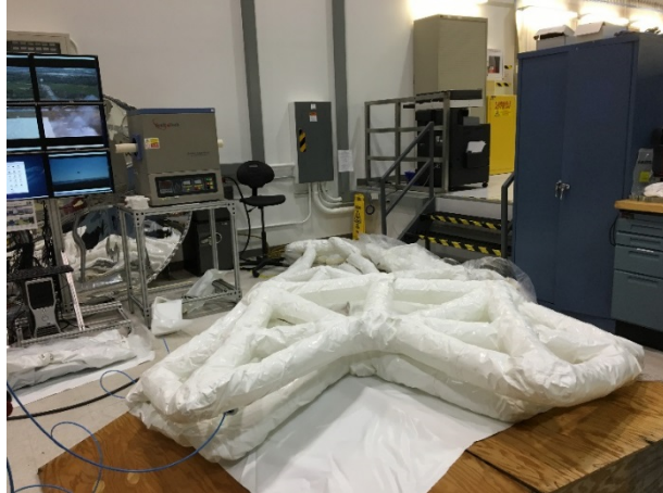
Figure 3.20. (Above) Tectoniks inflatable TransFormer scaled prototype in its deflated configuration in the NASA KSC Swamp Works Laboratory.
