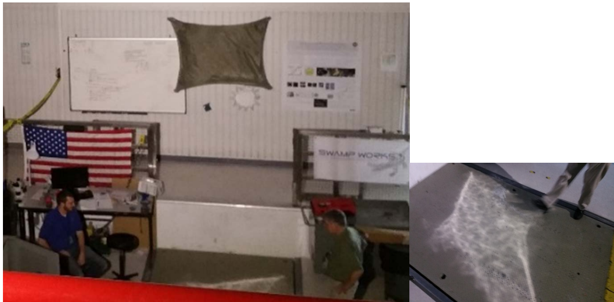
Figure 3.23. TransFormer reflectance testing. An LED array is shown reflected by a wrinkled Mylar sheet onto a laboratory floor.
