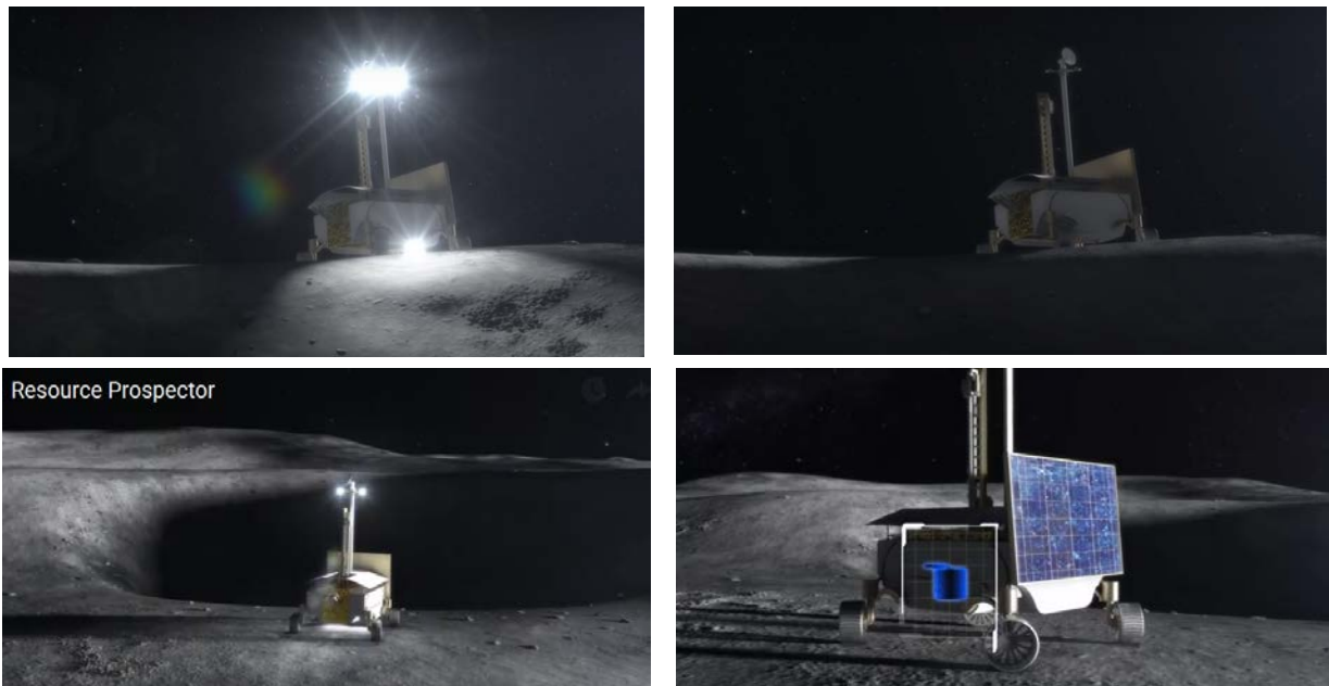
Figure 2.6. Illustration of Resource Prospector rover. The rover probes and analyzes soil, searching for water. Unfortunately, it is designed for operation in lunar daytime (under solar illumination) only. (Credit: NASA)
