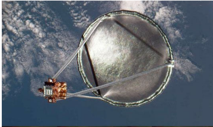
Figure 3.14. Deployed reflector with inflatable rigidizable torus along perimeter by L'Garde.
