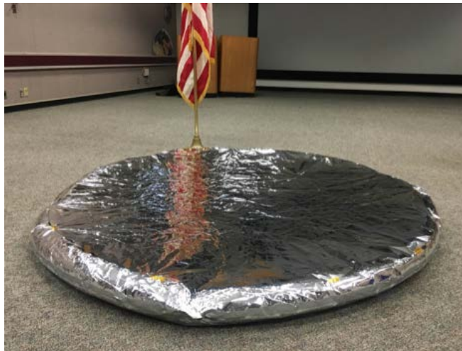
Figure 3.15. Deployable Mylar sheet with inflatable Mylar and vinyl torus; 2-meter diameter.
