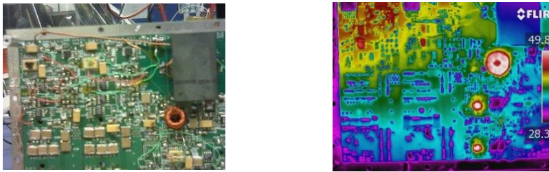
Figure 8. Left: Image of Board #2; Right: Thermal Image of Powered Board #2
