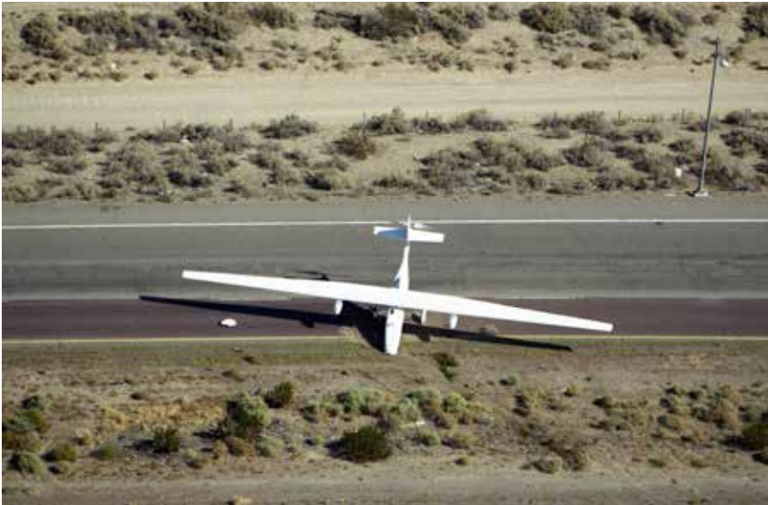
Failure of the flight-termination system led to an unplanned landing of Perseus-B on a major highway. NASA
