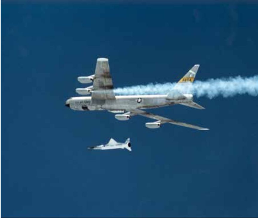
The X-43A-HXLV stack drops away from the B-52 over the Pacific Missile Range. NASA
