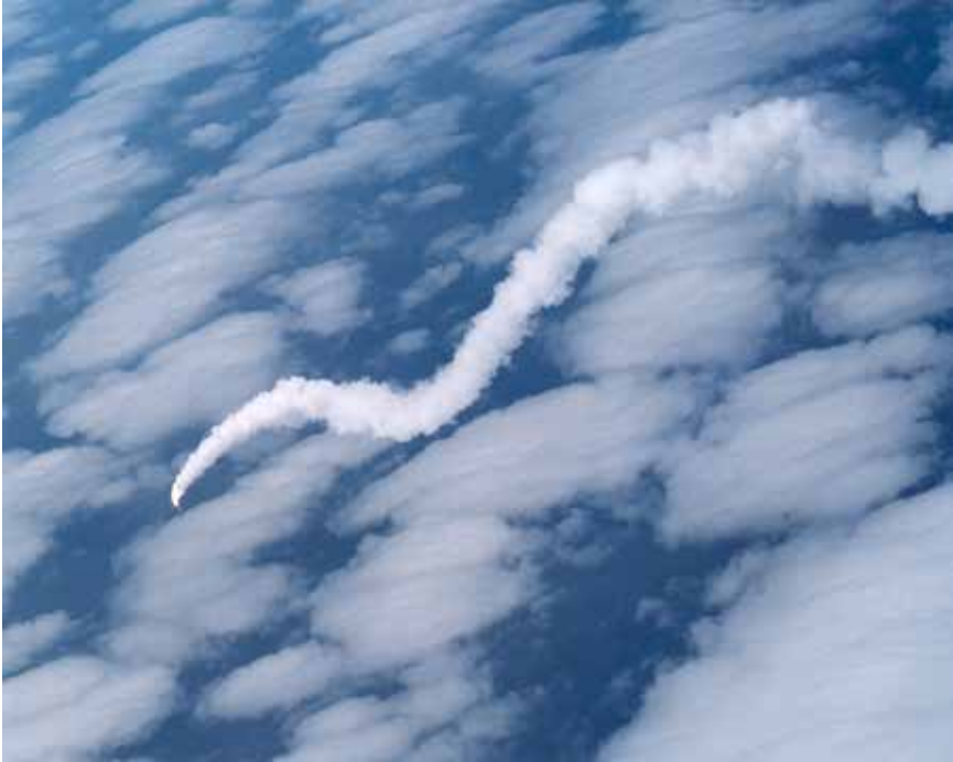
Divergent roll oscillatory motion caused by excessive control-system gain resulted from inadequate analytical modeling that allowed engineers to overestimate system safety margins. NASA
