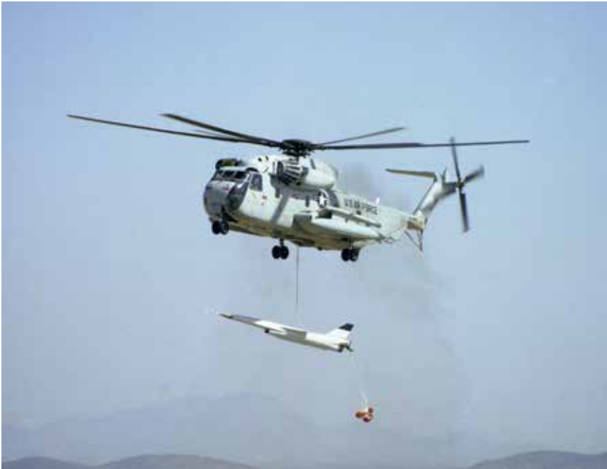
The DAST-1 vehicle is seen here following a typical MARS recovery. NASA
