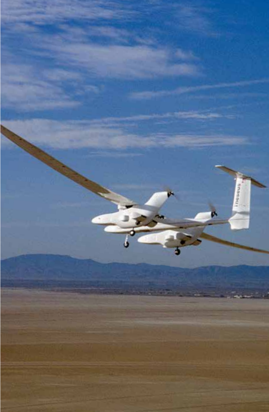
Initial flights of the Theseus demonstrated basic handling qualities at low and medium altitudes. NASA
