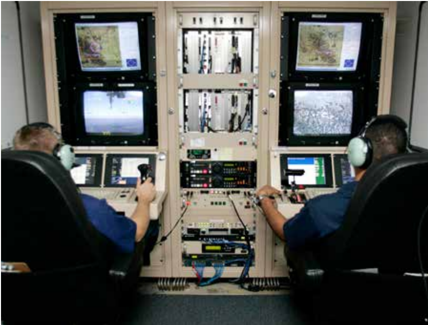
CBP agents operated the MQ-9 from a standard GCS, with identical consoles for pilot and sensor operator. CBP
