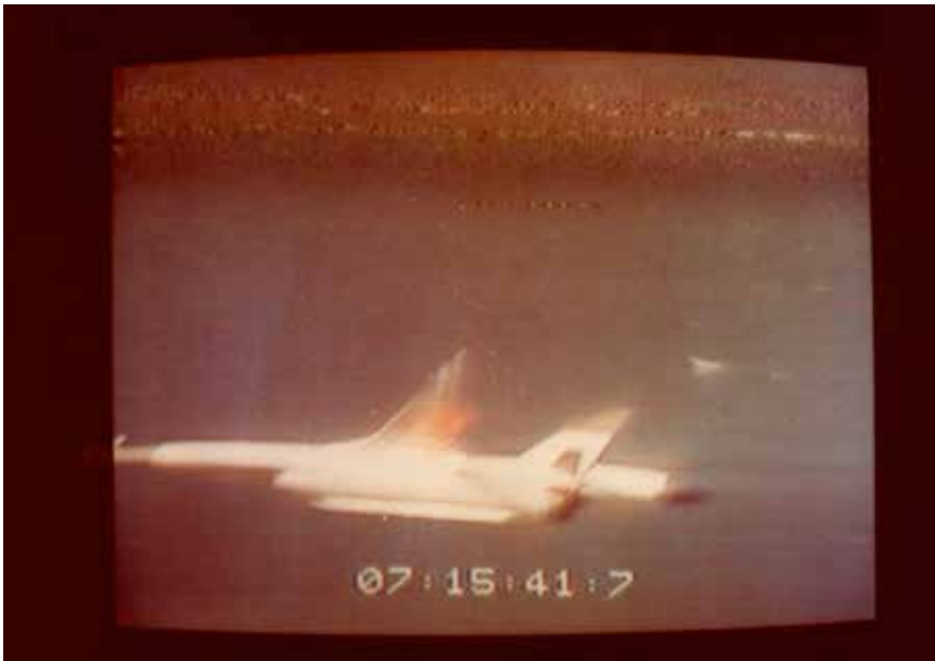
The DAST-1 experienced explosive flutter at Mach 0.825, leading to catastrophic failure of the right wing. NASA
