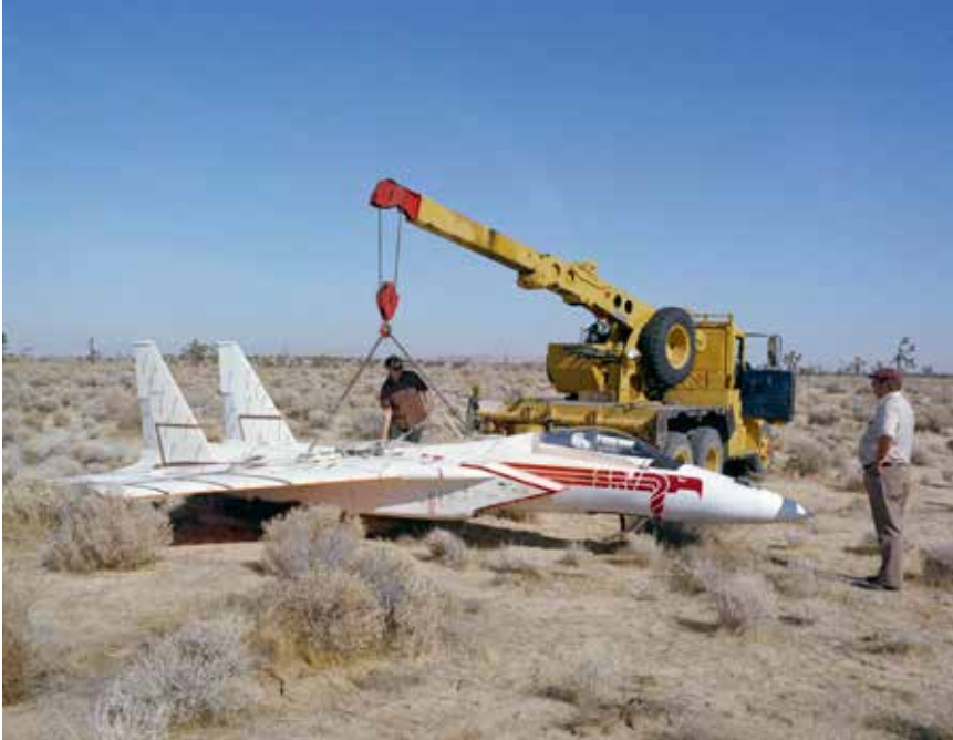
Recovery personnel prepare to lift the F-15 SRV off the Edwards Air Force Base PIRA after the vehicle's spin chute became entangled with the pitot tube. NASA
