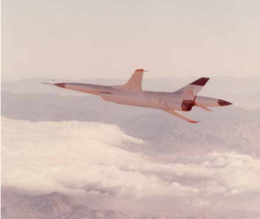
NASA researchers modified a Firebee II target drone, designated DAST-1, with supercritical wings of a shape optimized for a near-supersonic transport-type aircraft. NASA
