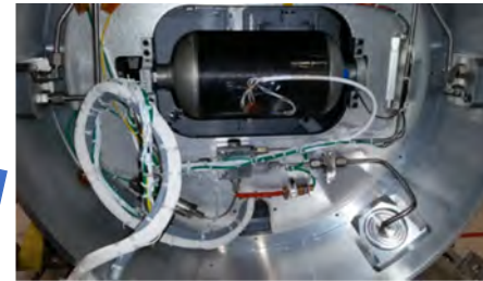
COPV Installed in Sounding Rocket Cold Gas Thruster System
