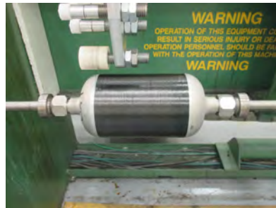
Filament Winding of Composite Overwrap Pressure Vessel (COPV)
