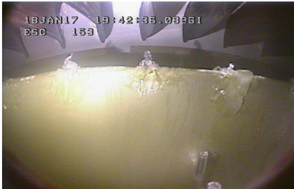
Figure 17.—Escort 153. Ice accretion with ice horns on the splitter.
