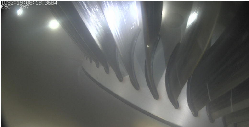
Figure 10.—Video camera view of the fan-stator showing that no ice accretion occurred there during Escort data 287.
