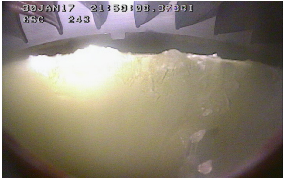
Figure 28.—Splitter-shroud: 5K altitude ice accretion on splitter-lip and shroud for Escort data point 243.
