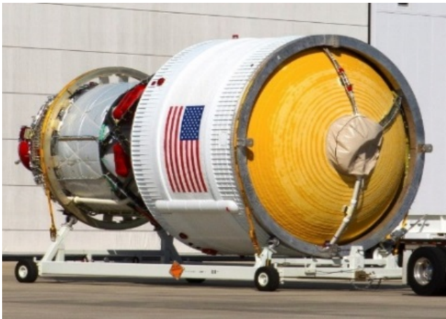
Fig. 12. The ICPS, which will provide in-space propulsion for the first integrated flight of SLS and Orion, is complete.
