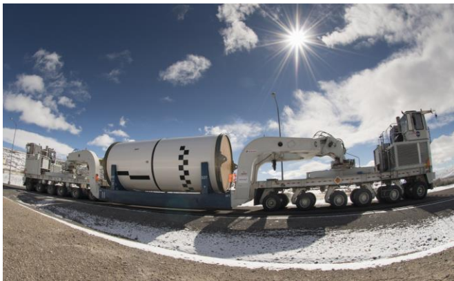
Figure 9. The 10 segments that will comprise the EM-1 motors are complete
