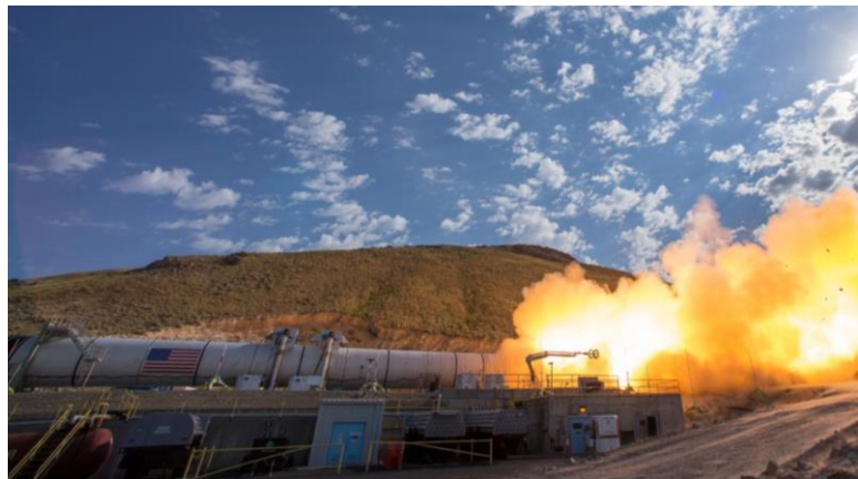
Figure 8. Five full-scale solid rocket motors have been test-fired to support flight certification
