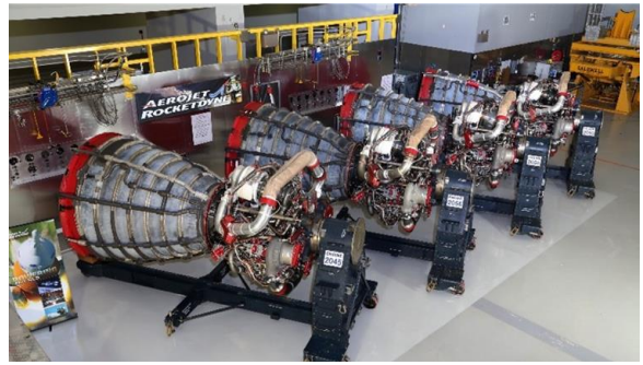
Figure 10. The four RS-25 engines for EM-1 are ready for integration with the core stage
