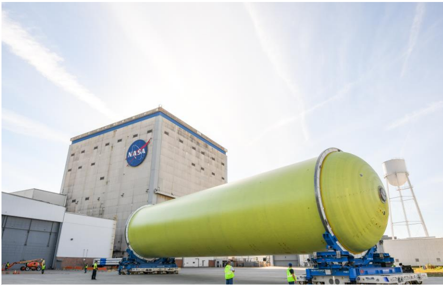
Figure 11. The EM-1 liquid hydrogen (LH2) tank under construction at Michoud Assembly Facility
