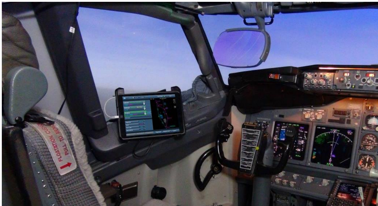
Figure 4. TAP software application displayed on the Alaska Airlines iPad EFB in a full-motion flight simulator. Photo credit: Janet Ann, Alaska Airlines.
