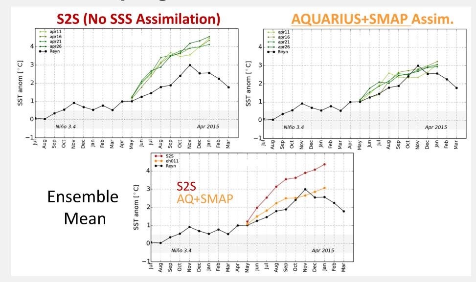
NINO3.4 forecast plume plots initialized from April 2015 for (top left) no SSS assimilation, (top right) assimilation of satellite SSS and (bottom) ensemble mean of Apr forecasts. Note that the thicker MLD from assimilation of SSS damps the warming of downwelling Kelvin waves for the big 2015 El Niño.
