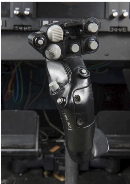
Figure 4. Center stick inceptor representative of OH-58D center stick.
