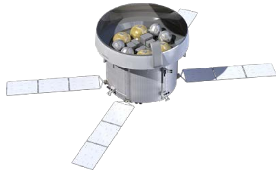
Figure 2. Overall view of the European Service Module (ESM).
