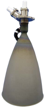
Figure 4. Aerojet R4D engine, similar to the ESM auxiliary thrusters.
