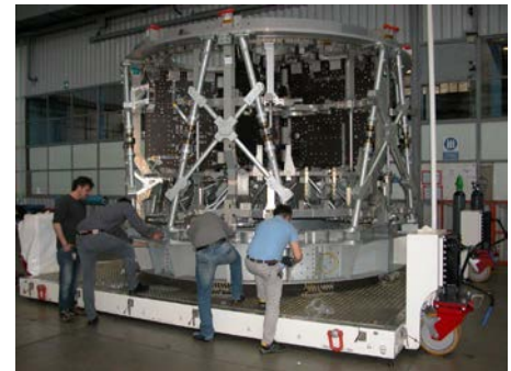
Figure 3. Primary structure of the ESM-2.
