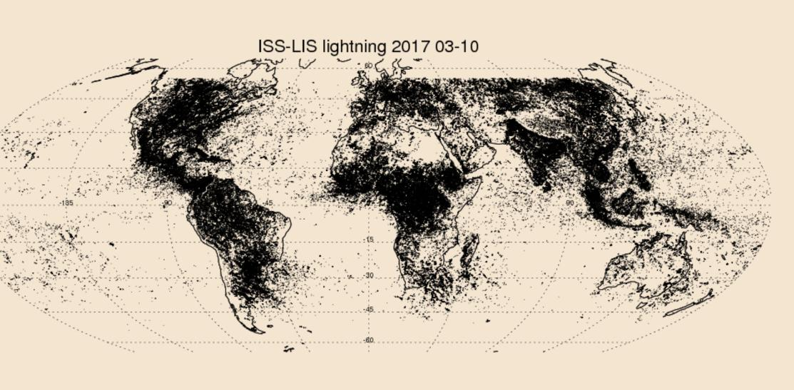
• Launched on February 19, 2017, the Lightning Imaging Sensor (LIS) instrument onboard International Space Station (ISS) is an instrument similar to the TRMM LIS. • Benefiting from ISS's 54° inclination orbit, the ISS-LIS provides a wider global coverage than the TRMM LIS and continues the long term optical observation of lightning since 1990s.
