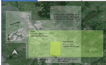
Figure 1: This figure demonstrates the satellite footprint size comparison between Aura/OMI and S5P/TROPOMI. The Airborne Prism Experiment (APEX) was an airborne flight campaign held in Antwerp, Brussels, and Liege in Belgium. TROPOMI's wide spectral coverage and the 3.5km by 7km spatial resolution bring space-based atmospheric chemistry remote sensing capability to a new, improved level.
