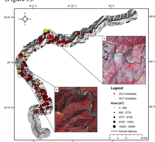
Figure 2. Location and area of landslides mapped along the Karnali highway for year 2012 and 2017. The insets show: (a) landslides mapped using QuickBird-2 imagery of 05/20/2013 and (b) landslides mapped using Sentinel-2A imagery of 11/10/2017. Imagery © 2013 DigitalGlobe, Inc.
