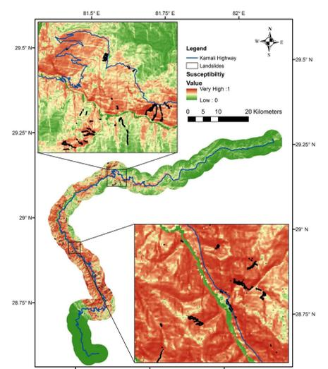
Figure 4. Landslide susceptibility map derived from logistic regression with inset plots highlighting two hazardous portions of the Karnali highway
