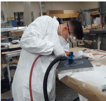
Figure 2a. Panel Scarfing. Pneumatic orbital hand sander and vacuum port used for scarfing.
