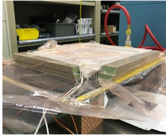
Figure 5. Cure Cycle. Panel was cured using hot bonder heater blanket
