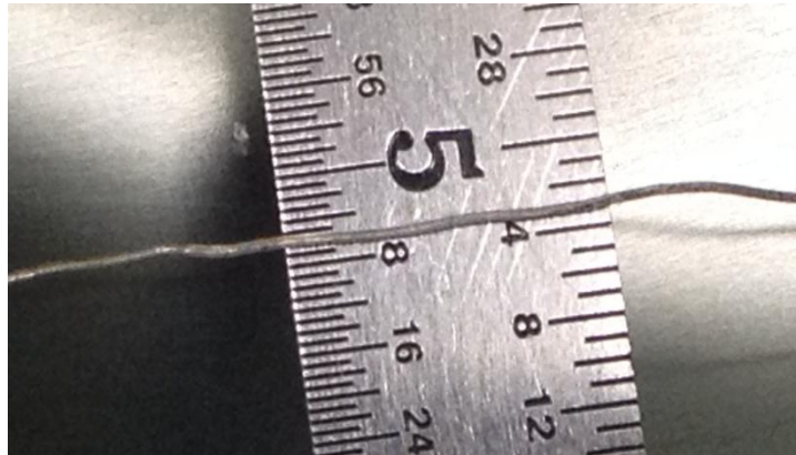
Figure 42 - Extruded wire, approximately 0.4mm (1/64") diameter.
