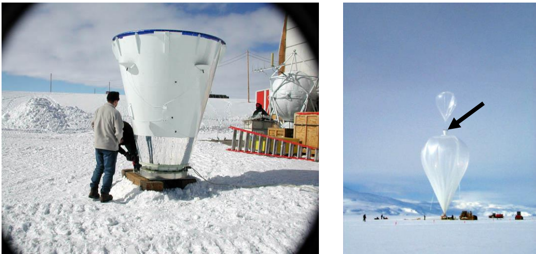
Figure V.F.2. TOPHAT payload prior to mating to balloon apex and after, with Tow balloon attached.
