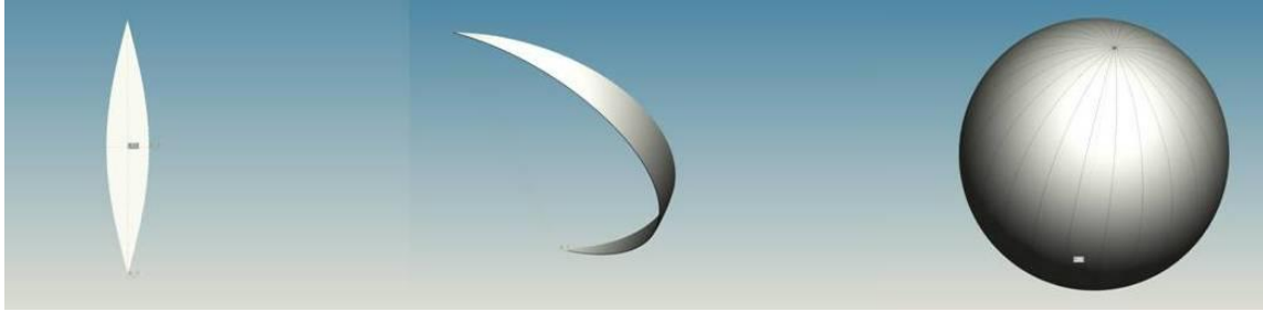
Figure V.B.3. Typical “gore” pattern sections used in most scientific balloons
