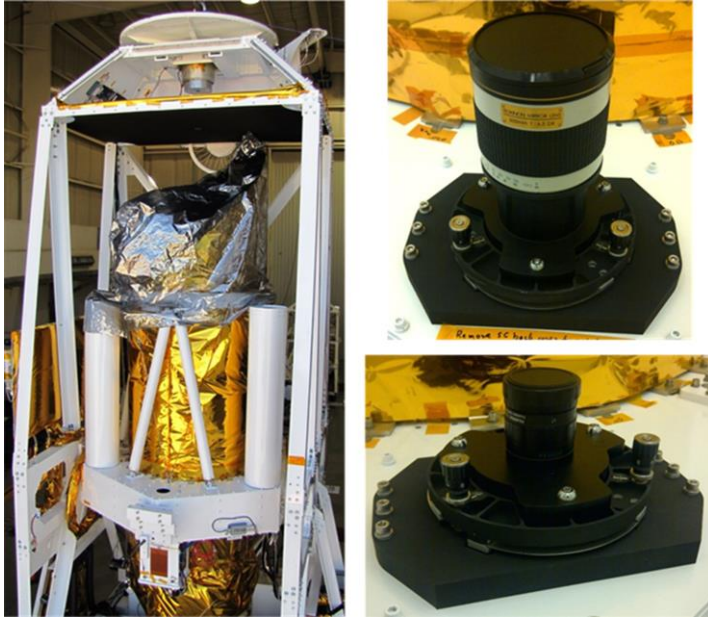
Figure V.D.2 Star Cameras installed on the BRRISON gondola. Left the 4.5 ft long baffles. Right top the NFC lens system. Right bottom the WFC lens system.
