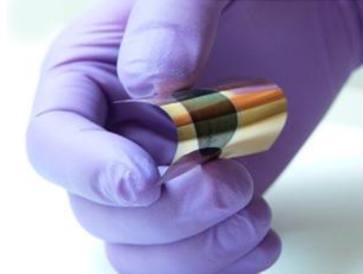
Figure 4.19. A thin film battery using a NiF 2 process [Yang2014].
