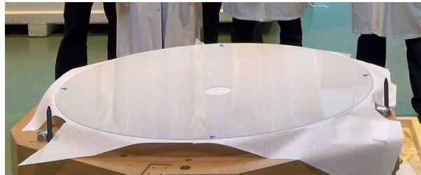
Figure 4.15. Thin-shell mirror made by SAGEM.
