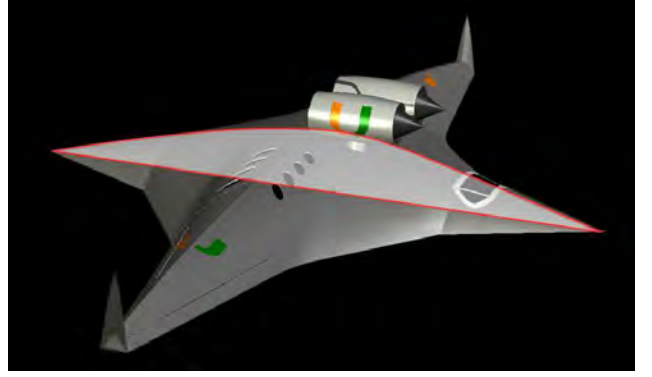
Figure 11: A SBiDir-FW civil transport in subsonic mode flying toward right, subsonic thick airfoil highlighted in the middle.
