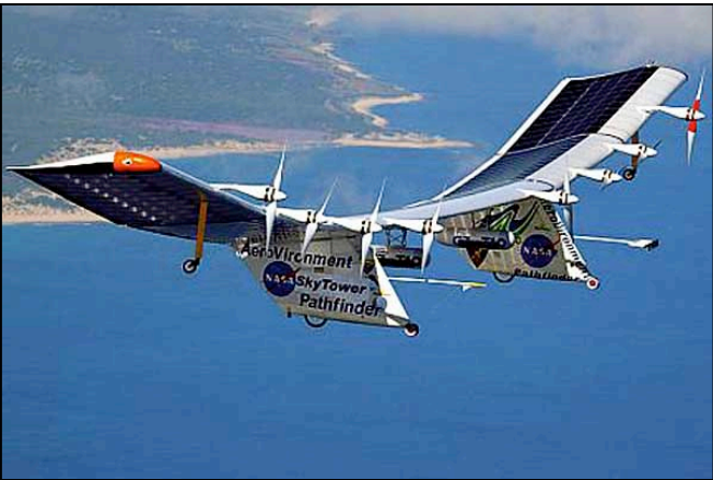
Solar-Battery Hybrid: NASA "Pathfinder"
