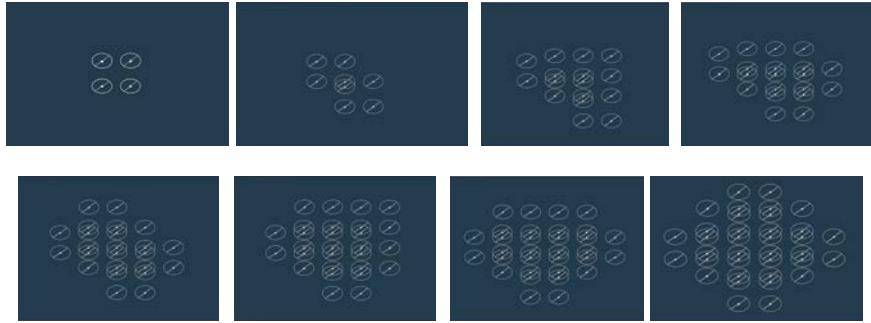
Figure 12 – Modular Configurations Comprised of “Stacked” Quadrotor “Building Blocks” (from four to thirty-six rotors)
