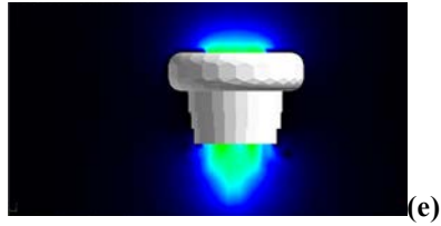
Figure 42 – Examples of Tailored-Contour Ducts/Shrouds for Multi-Rotor Vehicles: collapsible duct throughout flight regime from (a) cruise forward flight slowing down to (e) hover
