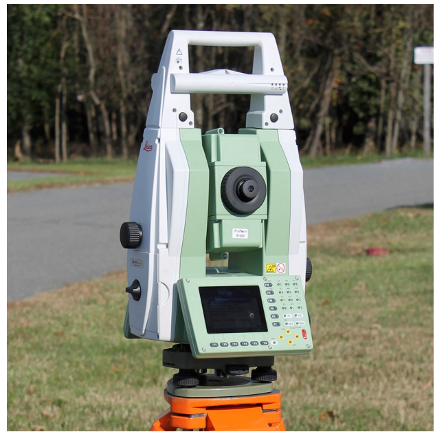
Fig. 5 Robotic Total Station (RTS) at GGAO that is part of the site's Vector Tie System (VTS)
