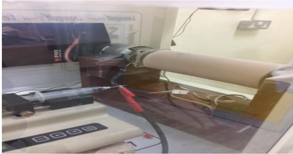
Figure 2.4. Fabrication of the fibers using electrospinning technique.
