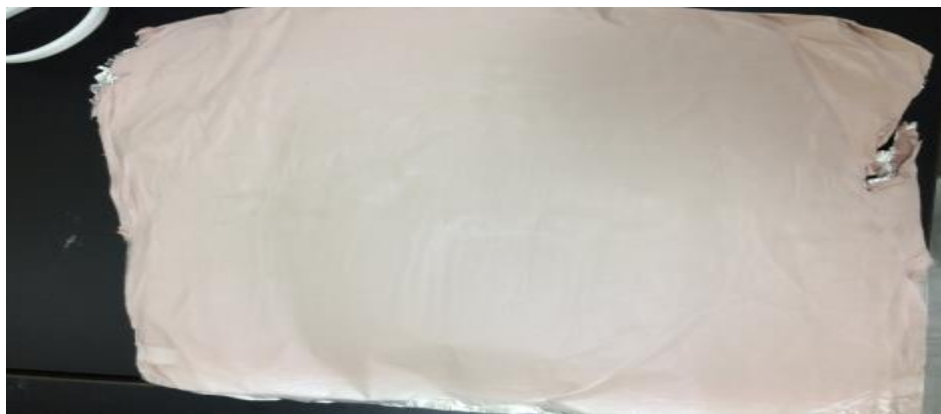
Figure 2.5. The produced fibers collected on the aluminum foil.
