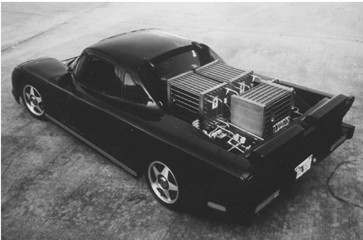
Figure 1.2. The first PEMFC powered passenger green car by Energy Partners, 1993 [4].
