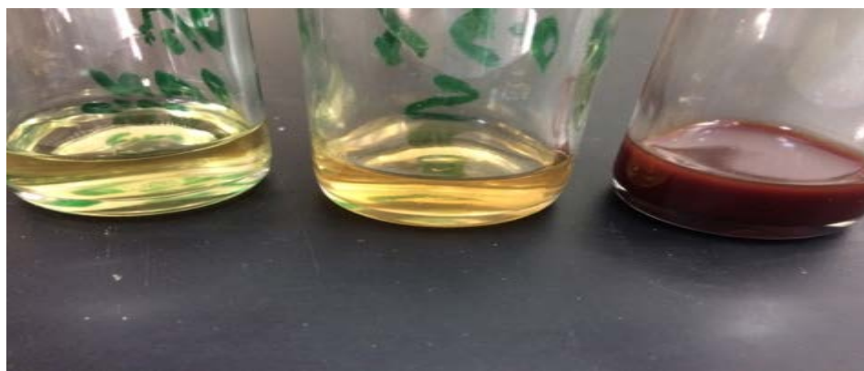
Figure 2.1. The prepared S-doped of PAN solutions with different sulfur sources.
