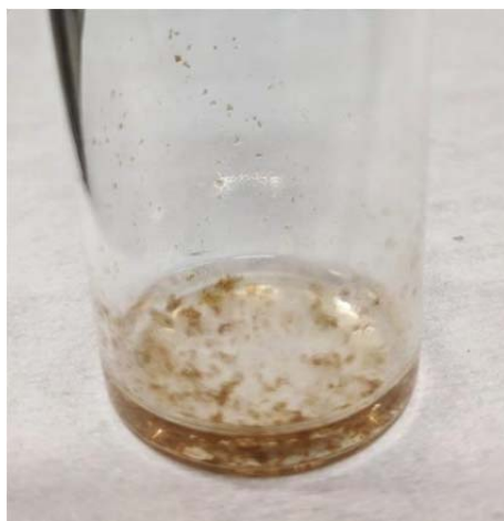
Figure 5.7. Precipitate formed in solution of 20 mM SP3 in THF containing 2:1 SP3: Co(NTf 2 ) 2 . Bright orange solution formed upon heating, and solid precipitated along with decoloration of the solution within several minutes upon cooling to room temperature.
