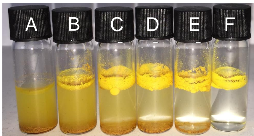
Figure 3.31. Photograph of ex situ synthesised mixtures LMWGs R 1 and R 6 suspended in water after 20 minutes of sonication. From left to right vials contain (in terms of LMWGs) A = 100% R 1 , B = 80% R 1 20% R 6 , C = 60% R 1 40% R 6 , D = 40% R 1 60% R 6 , E = 20% R 1 80% R 6 , and F = 100%.
