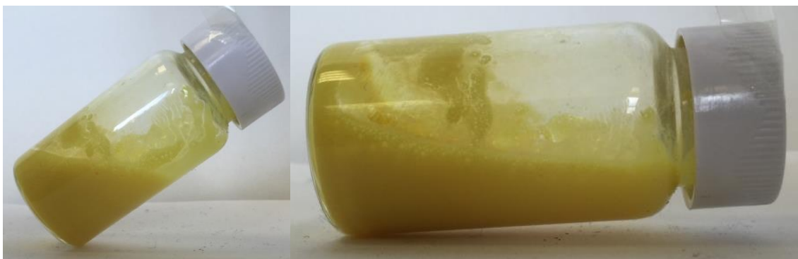
Figure 2.46. The suspension that arises from the in situ preparation of ligand C_{eB} in solution at pH 8, followed by the addition of GdL after a reaction time of four hours.
