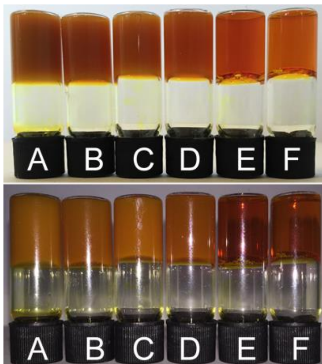
Figure 3.32. Photograph of gels composed of ex situ synthesised samples LMWGs R 1 and R 6 in various ratios. Gels set from suspensions shown in Figure 3.31 through the addition of sodium hydroxide up to a pH of 8, before the addition of 9 equivalents of GdL. From left to right vials contain (in terms of LMWGs) A = 100% R 1 , B = 80% R 1 20% R 6 , C = 60% R 1 40% R 6 , D = 40% R 1 60% R 6 , E = 20% R 1 80% R 6 , F = 100%.
