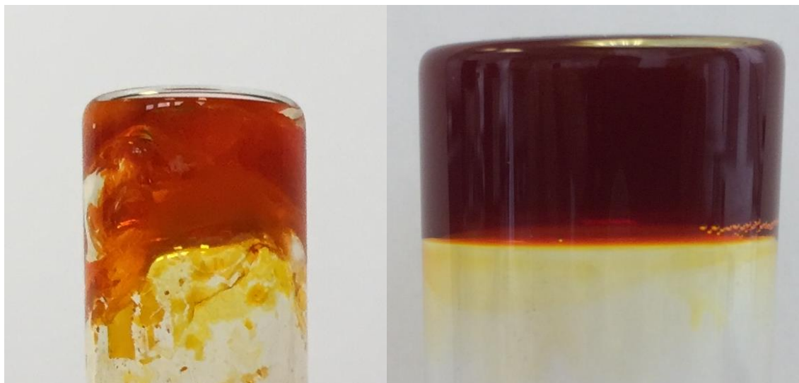
Figure 2.4. Close up photograph of gel set using concentrated HCl (left) and set with GdL (right). The differences in homogeneity are apparent with the GdL set gel having a highly uniform structure, when compared with the HCl set gel.
