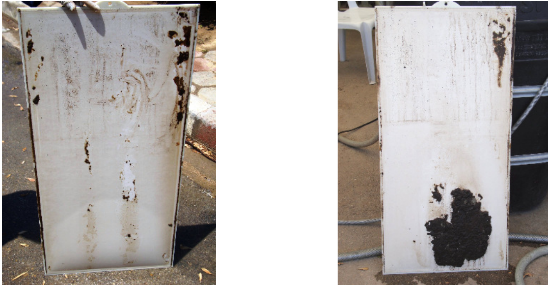
Figure 6.41 MBR1: Irreversible membrane fouling
