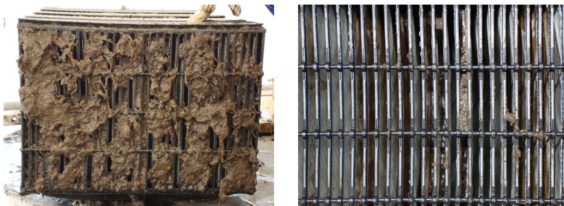
Figure 6.43 MBR3: Irreversible membrane fouling
