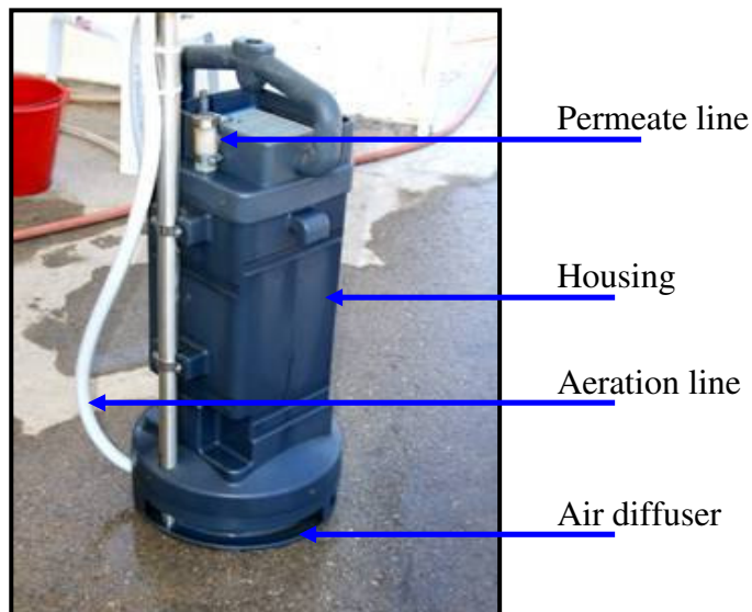
Figure 3.10 MBR2: Membrane unit, its housing and the diffuser
