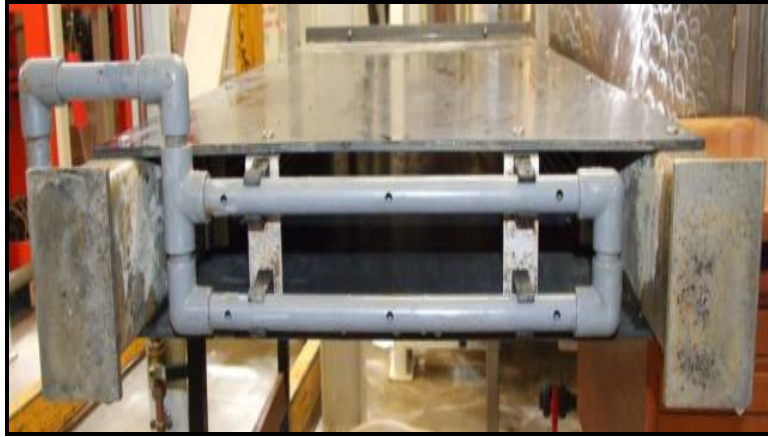
Figure 3.5 MBR1: Air diffuser
