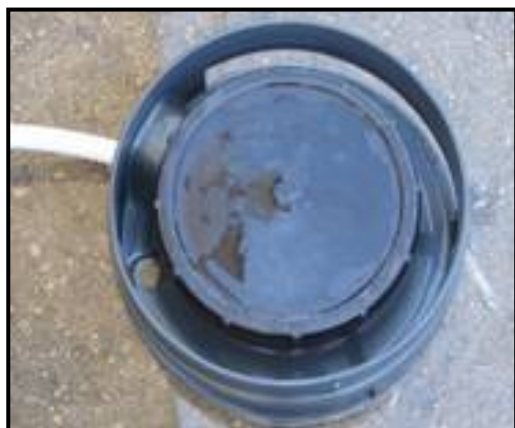
Figure 3.9 MBR2: Air diffuser
