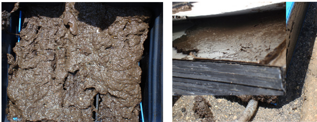
Figure 6.42 MBR2: Irreversible membrane fouling
